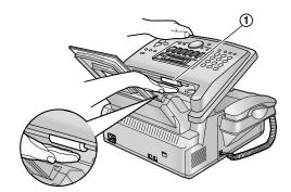
4 Hold the centre part of the front cover (1), and pull open the inner cover (2).
